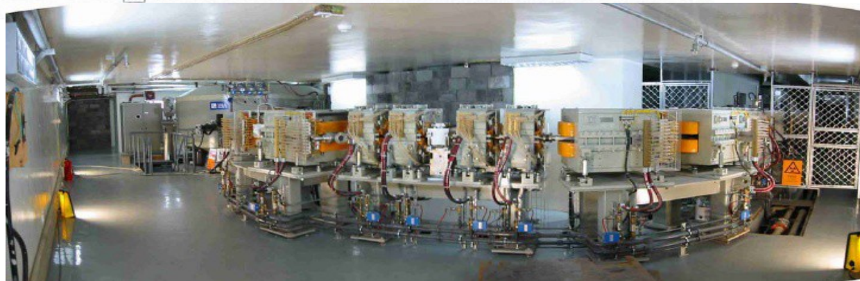
Set of slits and magnets for monochromatization of the scattered beam
