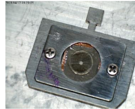
{}^{254}\text{Es} Target (10 ng on \Phi 2\text{mm} )
