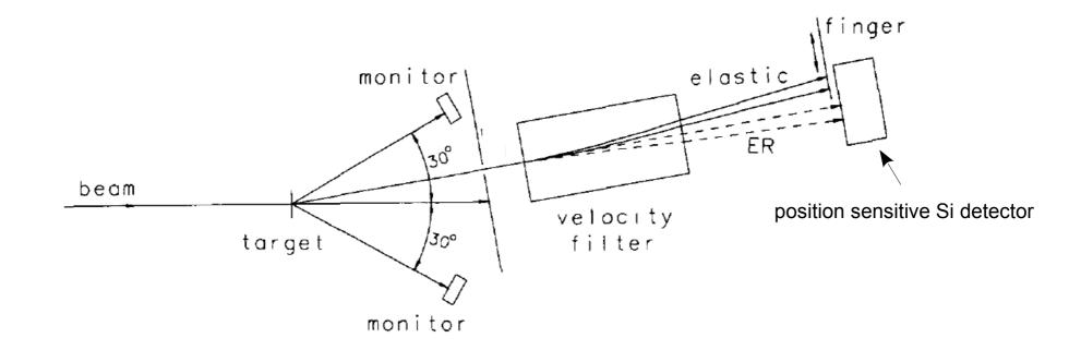
• direct measurements of  $\sigma_{fus}(E)$  and  $D_{fus}$
