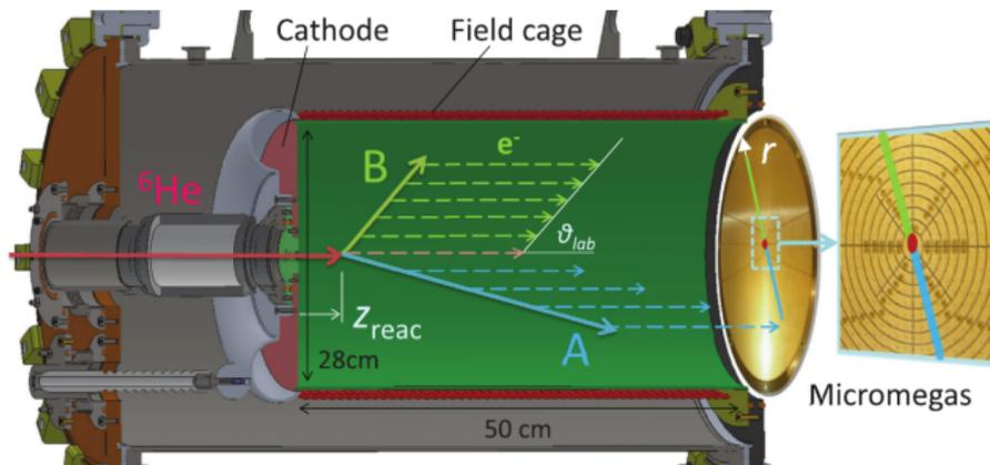
Figure 5: AT-TPC operating principle. [1])
