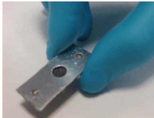
Self-supported Si:He target
