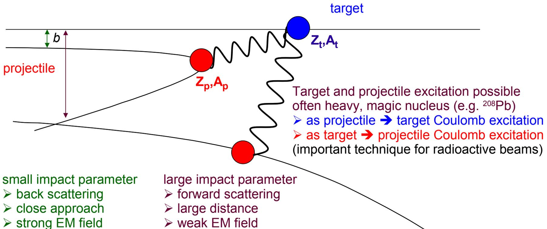
Coulomb trajectories only if the colliding nuclei **do not reach the "Coulomb barrier"** → purely electromagnetic process, no nuclear interaction, calculable with high precision
