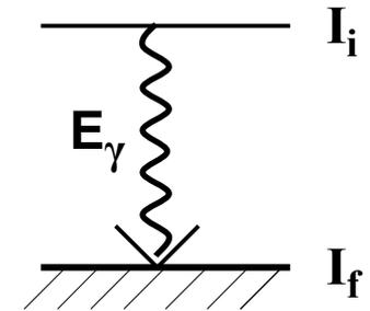
Calculation includes effects influencing  $\gamma$ -ray intensities: **internal conversion, size of Ge,  $\gamma$ -ray angular distribution, deorientation**
