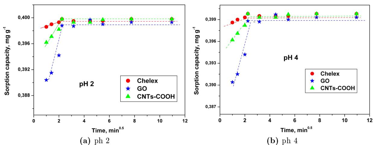
**Figure 2:** Intra-particle diffusion plots for graphene oxide, carbon nanotubes and Chelex 100 resin.
