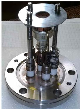
**Figure 2:** Prototype of thermal lithium  $1^+$  ion source.
