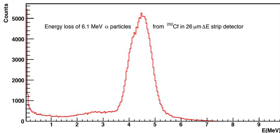
Figure 1: Energy loss of 6.1 MeV  $\alpha$  particles from  $^{252}\text{Cf}$  in the  $\Delta E$  detector.
