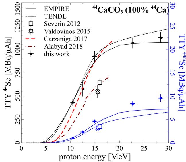
Figure 2: Thick target yields for  $^{44}\text{Sc}$  and  $^{44\text{m}}\text{Sc}$  production with proton projectiles.
