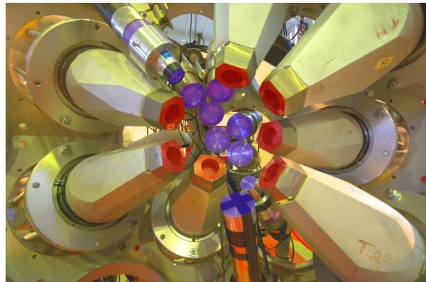
**Figure 1:** The first stage of the EAGLE-EYE setup with 10 LaBr detectors marked in blue. HPGe spectrometers are marked in red.
