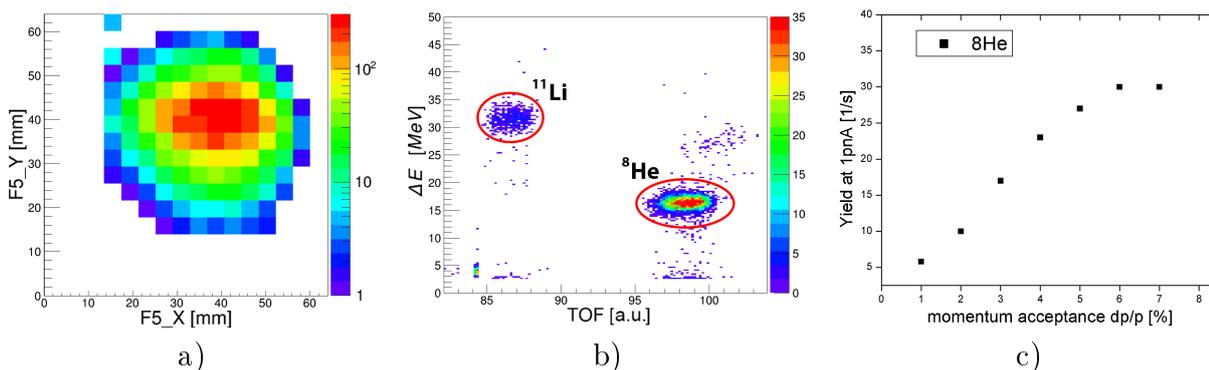
**Figure 2:** Typical spectra for the settings on  $^8\text{He}$ . a) XY profile at the F5 focal plane obtained by a double-sided Si strip detector. b)  $\Delta E$  vs. TOF fragment identification spectra. c) Dependence of the  $^8\text{He}$  yield on the momentum acceptance of ACCULINNA-2 measured in the focal plane F5. Measurements were performed with a 1 mm beryllium wedge and  $\Delta p/p = \pm 2\%$  at F2,  $B\rho(D2) = 2.67 \text{ Tm}$ .
