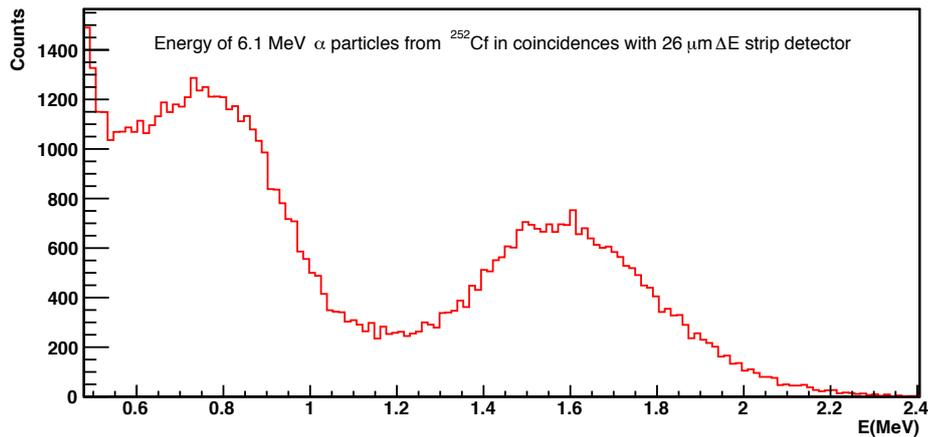
Figure 2: Energy of  $\alpha$  particles stopped in a strip of the E detector.
