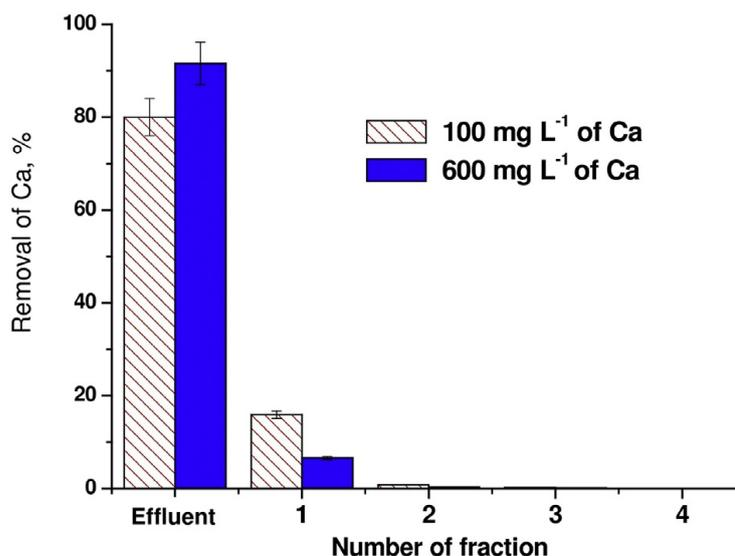
**Figure 2:** Removal of  $\text{Ca(II)}$  by the use of CNTs from mixtures containing calcium at concentrations of 100 mg/l or 600 mg/l.
