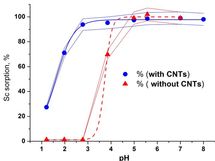
**Figure 1:** The effect of pH and precipitation on Sc(III) removal with and without CNTs.
