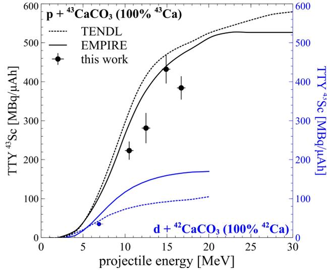
Figure 1: Thick target yields for  $^{43}\text{Sc}$  production with proton and deuteron projectiles.
