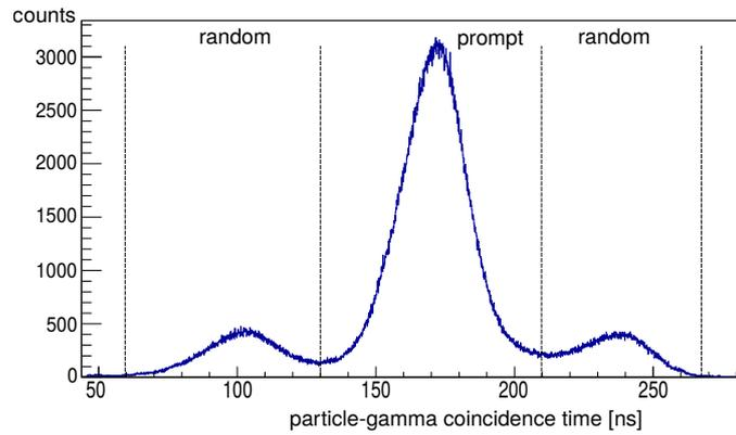
**Figure 1:** The particle- $\gamma$  coincidence spectrum collected by one of the germanium detectors in the  $^{32}\text{S}+^{107}\text{Ag}$  Coulomb excitation experiment. Prompt and random coincidence gates are marked.
