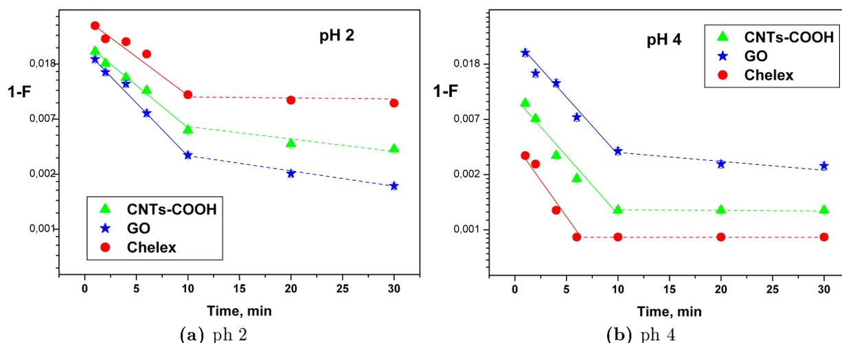
**Figure 1:** Fractional attainment for Sc(III) sorption by different sorbents.
