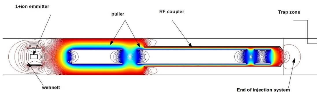
**Figure 3:** Equipotential lines for the  $1^+$  injection system mounted in the extension of the plasma chamber. Two gaps in the puller (extraction electrode from the  $1^+$  source) give a better optical condition of the incoming beam.
