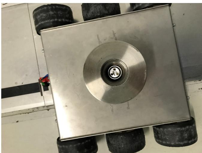
**Figure 3:** An irradiated target inside a lead container placed on a remotely controlled trolley.
