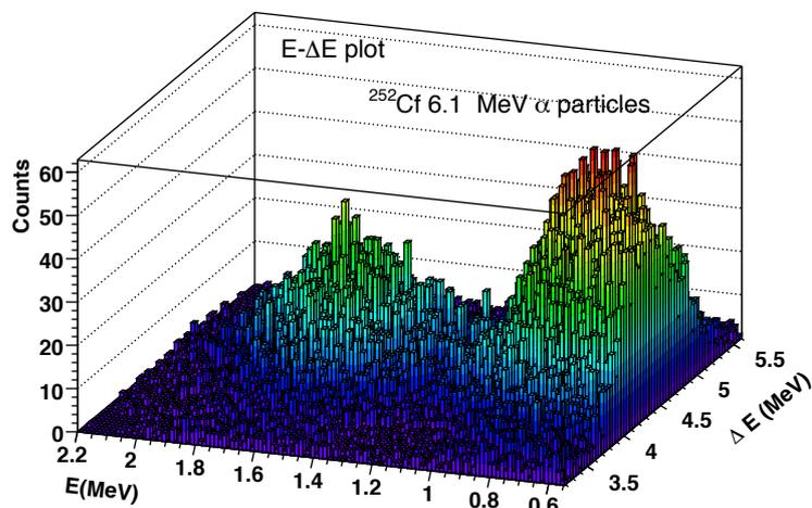
Figure 3: Two-dimensional spectrum of 6.1 MeV  $\alpha$  particles registered in the  $\Delta E - E$  telescope.
