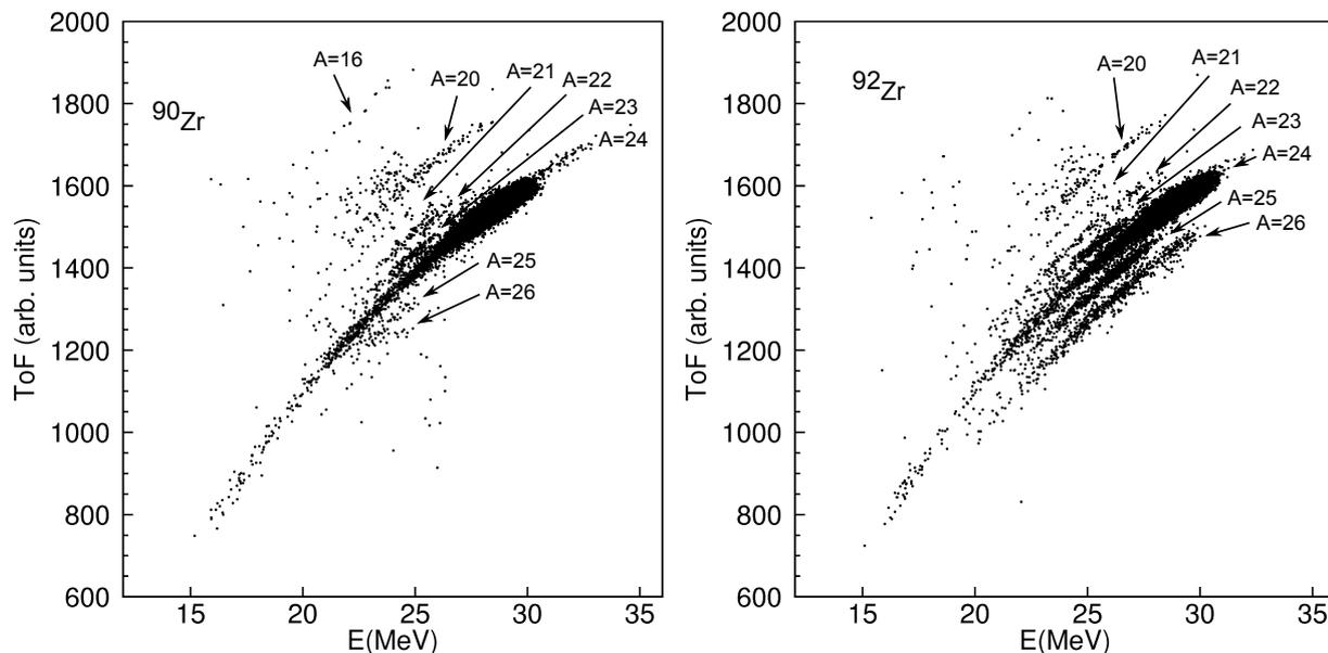
**Figure 1:** The raw E-ToF spectra of back-scattered ions, measured at  $\theta_{lab} = 142.5^\circ$  for the  $^{24}\text{Mg} + ^{90}\text{Zr}$  (left panel) and  $^{24}\text{Mg} + ^{92}\text{Zr}$  (right panel) systems.
