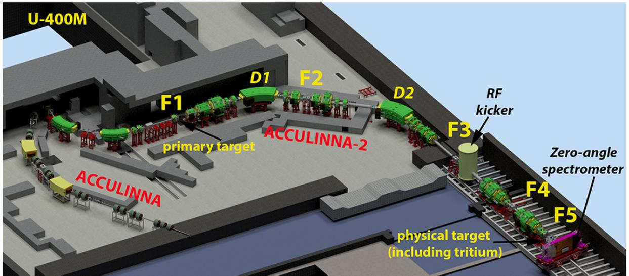
**Figure 1:** Layout of the ACCULINNA-2 fragment separator at the U-400M cyclotron. The 5 separator focal planes are indicated by F1 to F5.
