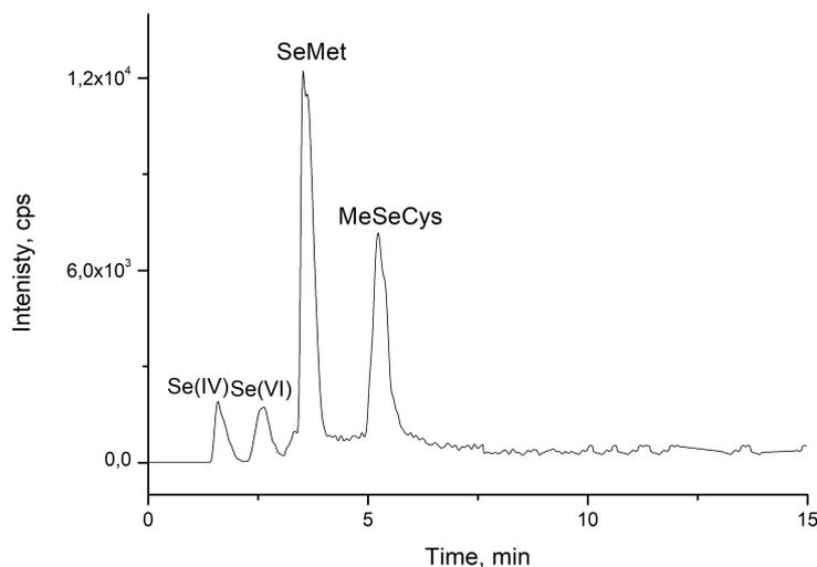
**Figure 1:** The chromatogram of extract from onion leaves supplemented with selenite. Column: Atlantis HILIC (silica), eluent: 85% methanol and 8 mM ammonium acetate, pH 7 (isocratic mode).
