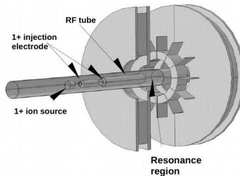
**Figure 1:** Schematic proposal for the  $1^+$  injection setup model.
