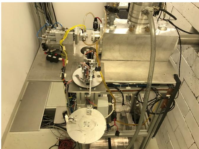
**Figure 2:** The standalone external target system with robot and carousel.
