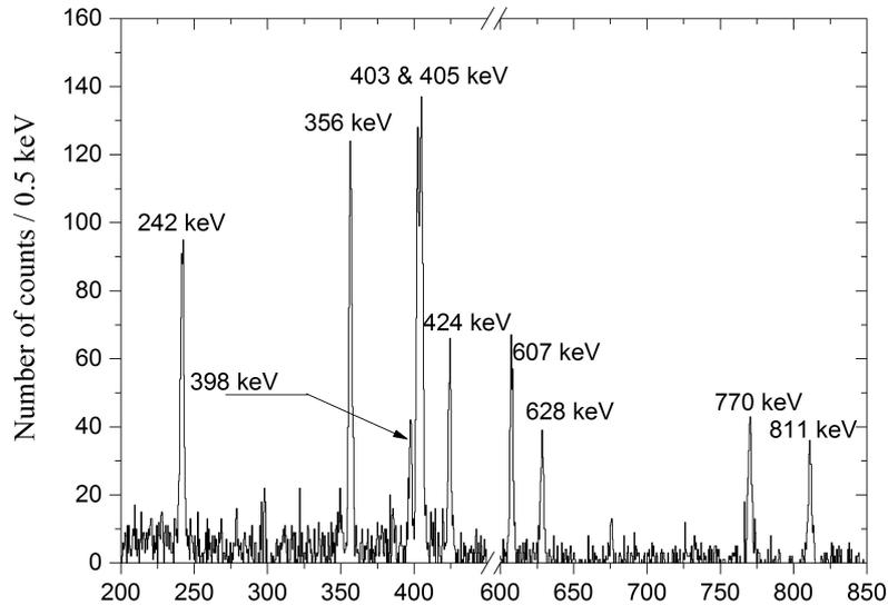
**Figure 1:** The coincidence gamma spectra with 403 and 405 keV transitions collected during two time spans after the end of the cyclotron beam pulse. The transitions from the decay of the  $I^\pi = K^\pi = 8^-$  isomeric states in  $^{186}\text{Hg}$  are labelled.
