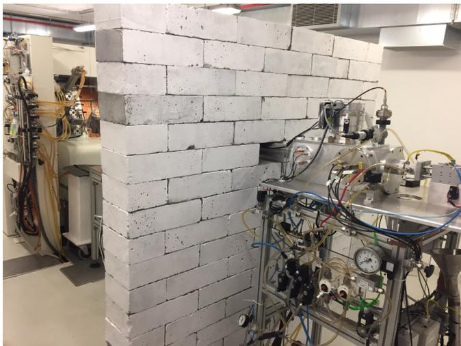
**Figure 1:** A view of the standalone external target system with the shielding wall and the cyclotron.
