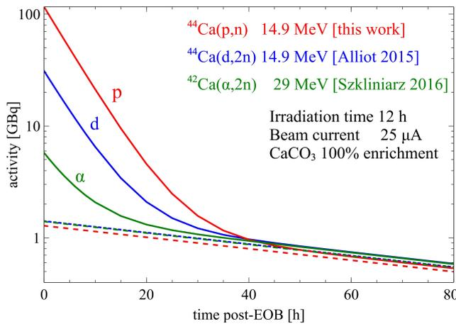
Figure 3: Calculated evolution of  $^{44\text{m}}\text{Sc}$  (dashed line) and  $^{44}\text{Sc}$  (solid line) activities after irradiation with different beams.
