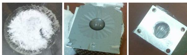
**Figure 3:** Crystals of Ba oxalate (left), solution of Ba-acetate on C foil (middle) and solution of Ba-acetate on Mylar (right)
