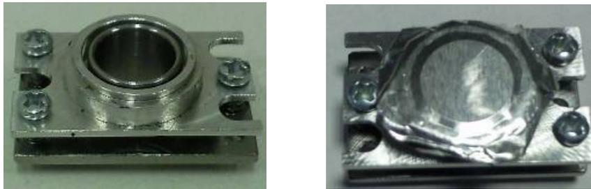
**Figure 1:** The plunger device: left showing the inside dome, right with stretched test foil.
