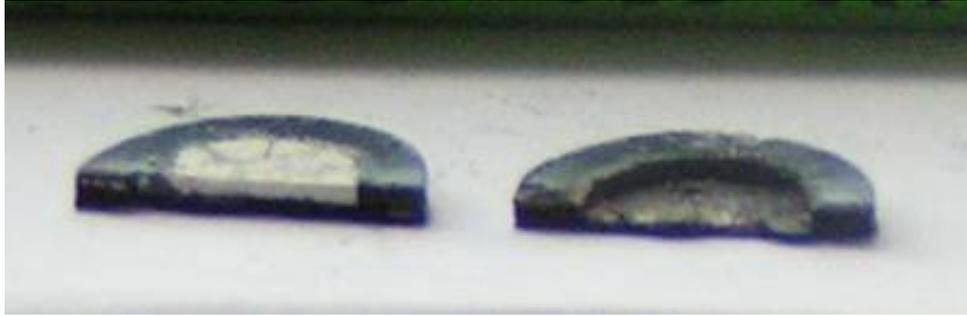
**Figure 2:** Cut through a 100 mg/cm<sup>2</sup> CaCO<sub>3</sub> target in graphite bed.
