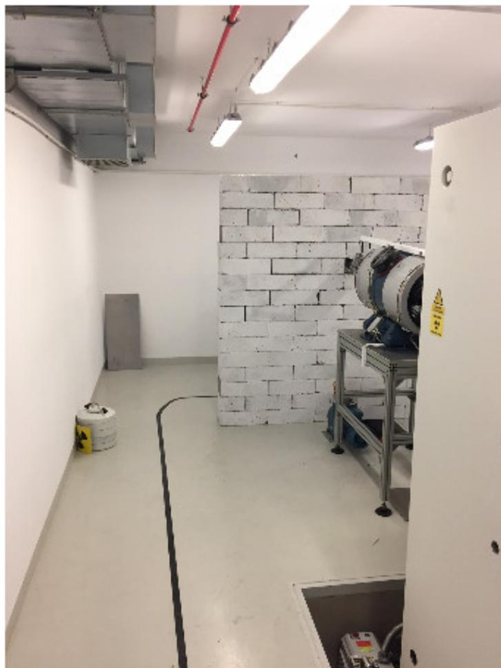
**Figure 2:** The modified beam line with shielding wall.
