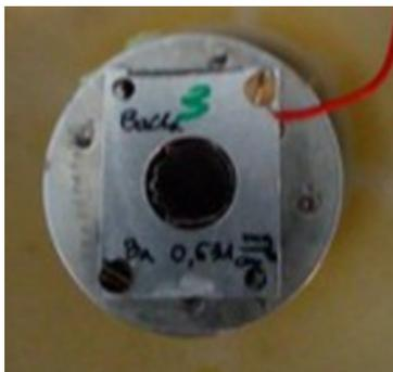
**Figure 2:**  $\text{BaCl}_2$  target mounted at a target holder.
