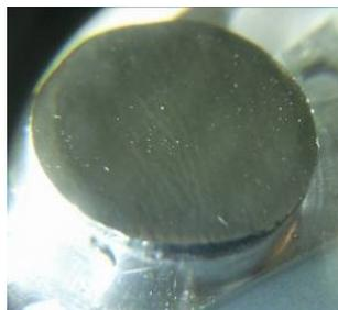
**Figure 4:** The test deposit of nat Sn on Al backing, the small droplets of Sn are visible on the surface (magnification: 40 times)
