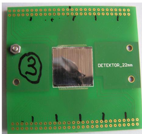
**Figure 2:** PCB with glued strip detector.
