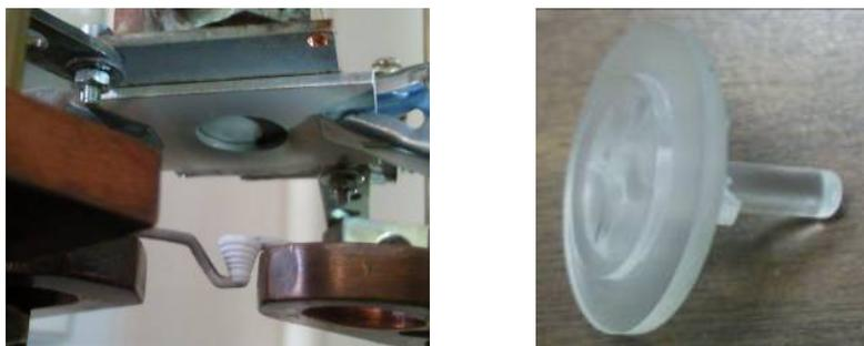
**Figure 3:** Evaporation set-up (left). The axial position of the crucible and backing foil was controlled with the tool shown on the right.
